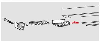
The **RF** mechanical hold-open unit ensures that doors are held open at precisely the correct angle – up to approx. 150° – without any fallback.
