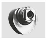
The heart-shaped cam and the linear drive mechanism which characterise all DORMA camaction door closers produce a rapidly decreasing opening torque, so greatly reducing the amount of effort required. This means that even children, the elderly and the disabled can open doors with ease. The user-friendliness of the system is further enhanced by the reliable latching action achieved by the fact that the closing force only rises in the end phase of the cycle.
