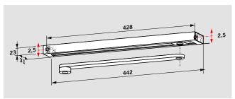
The **G-N** slide channel assembly comprises the main arm, slide channel, slide block, fixings, screws and end caps. The G-N slide channel is non-handed and can be combined with both door closers
